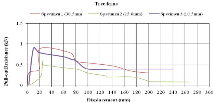
Figure 4. Plots of pull-out resistance against displacement for Tree ferns (*Asparagus species*)
