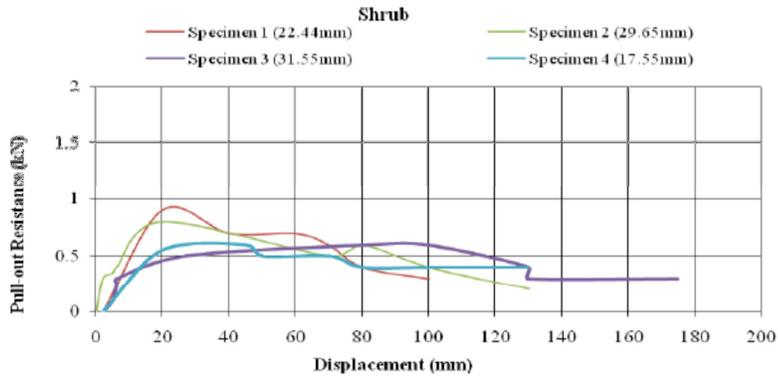
Figure 2. Plots of pull-out resistance against displacement for Saltbush (*Atriplex halimus*)
