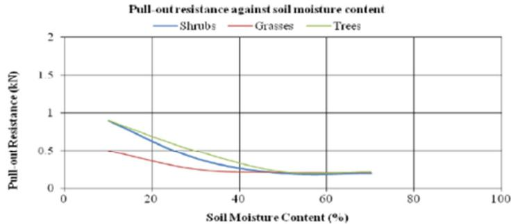
Figure 5. Plots of pull-out resistance against soil moisture content
