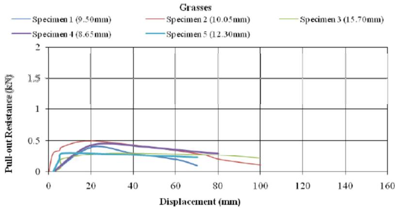
Figure 3. Plots of pull-out resistance against displacement for Switch grass (*Panicum virgatum*)
