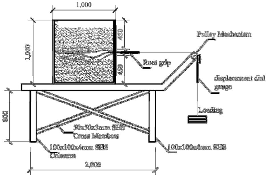
Figure 1. The Pull-out test Apparatus
