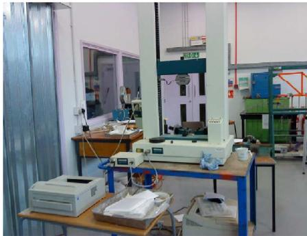
Figure. 2: The 50kN Universal Testing Equipment assembly
