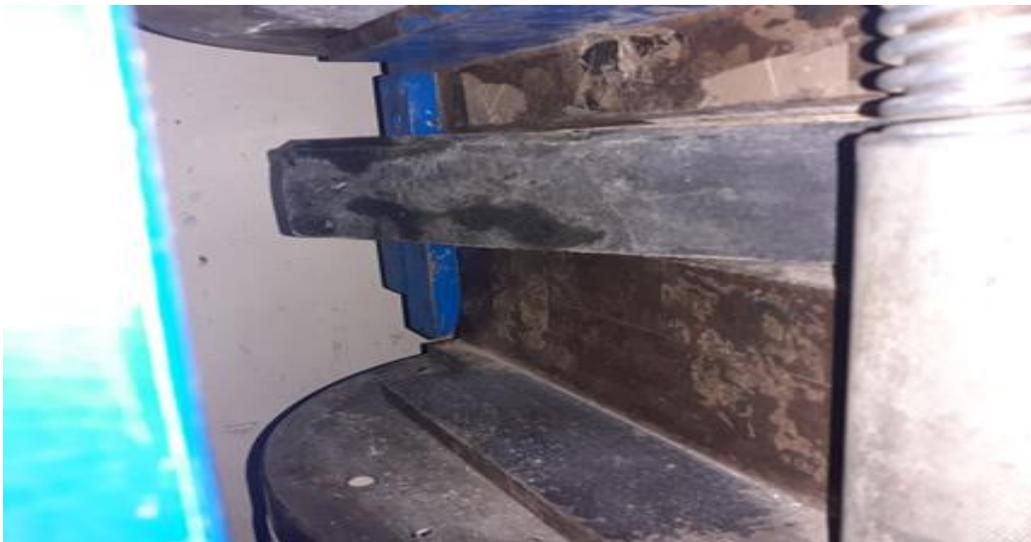
The area of failure,  $S$  ( $\text{mm}^2$ ) was then obtained by multiplying the mean of the two measurements of
