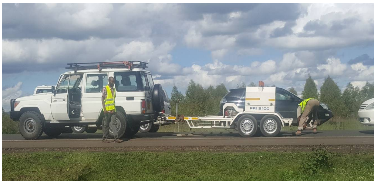
Plate 1: Pavement Surface Deflection Measurement Using FWD Equipment
