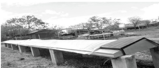
Fig. 1. Pictorial view of the solar tunnel dryer from the collector end.
