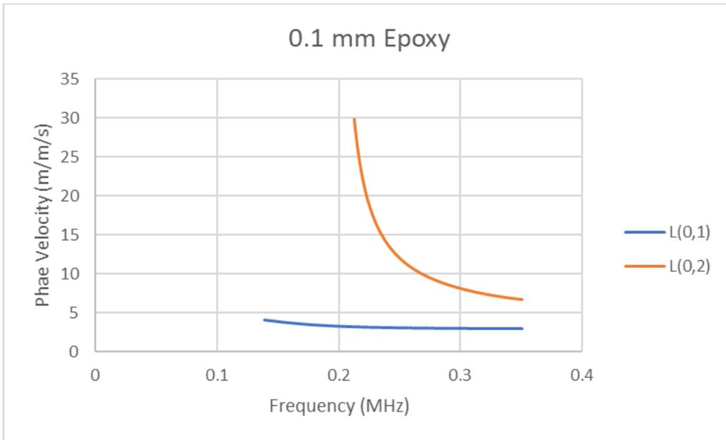
Figure 4: Disperse plot for Rebar in concrete with 0.1mm epoxy layer
