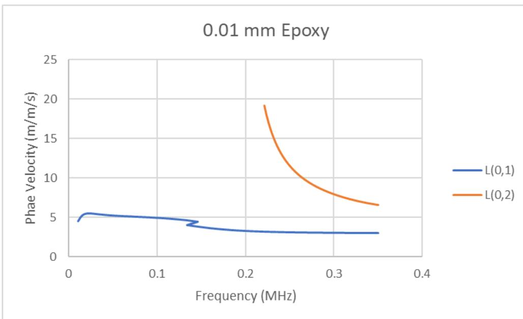
Figure 5: Disperse plot for Rebar in concrete with 0.01mm epoxy layer
