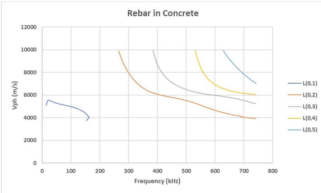
Figure 2:: Disperse plot for Rebar in Infinite Concrete
