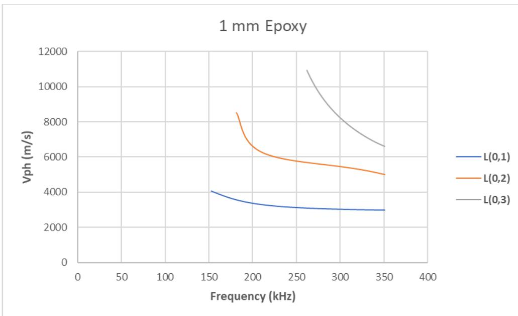
Figure 3: Disperse plot for Rebar in concrete with 1mm epoxy layer
