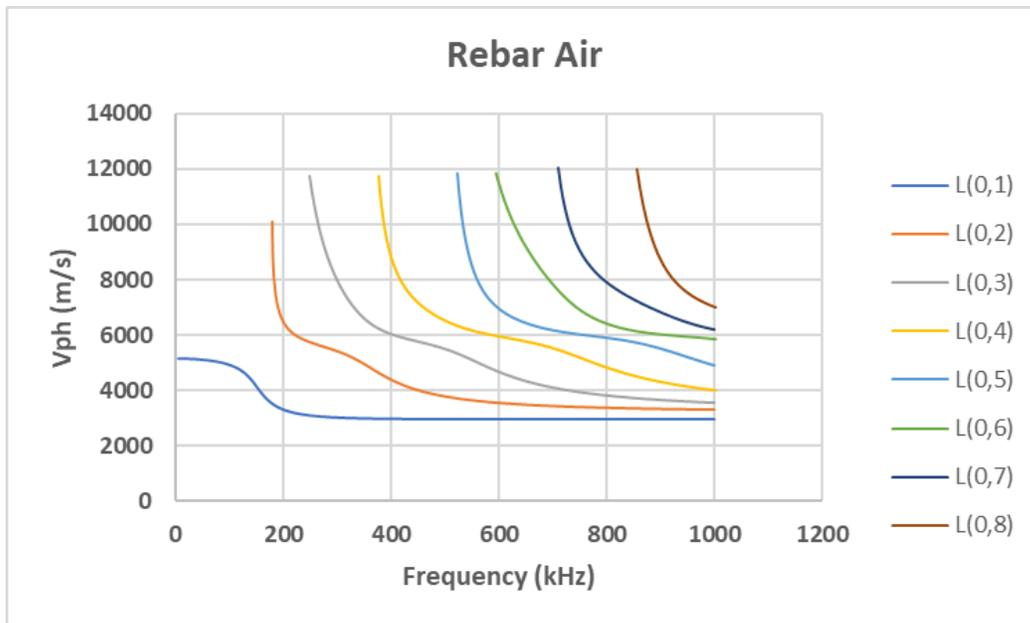
Figure 1: Disperse plot for Rebar in Air
