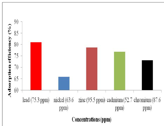
Figure 5: Efficiency of water hyacinth powder in the removal of heavy metals from aqueous solution.
