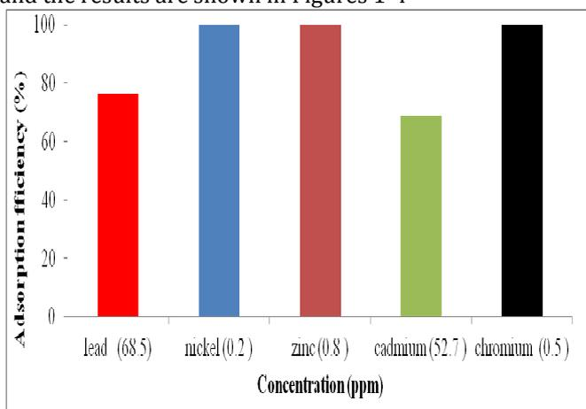
Figure 1: The effects of powdered water hyacinth on the concentration of heavy metals in wastewater collected from site A (Battery manufacturing Company)
