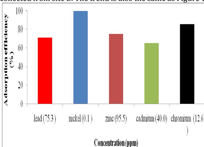
Figure 2: The effects of powdered water hyacinth (<300 μm) on the concentration of heavy metals in waste-water collected from site B (Paints manufacturing Company)
