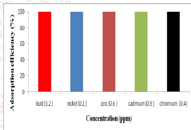
Figure 4: The effects of powdered water hyacinth (<300 μm) on the concentration of heavy metals in waste-water collected from site D (Plastic manufacturing Company).
