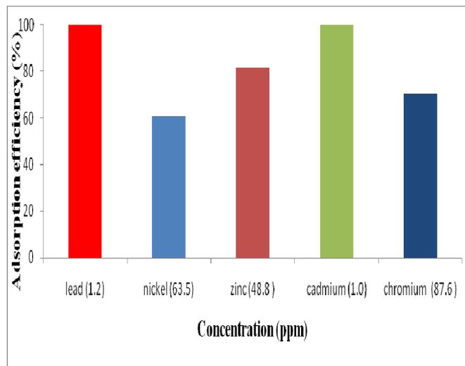
Figure 3: The effects of powdered water hyacinth (<300 μm) on the concentration of heavy metals in waste-water collected from site C (Steel manufacturing Company).
