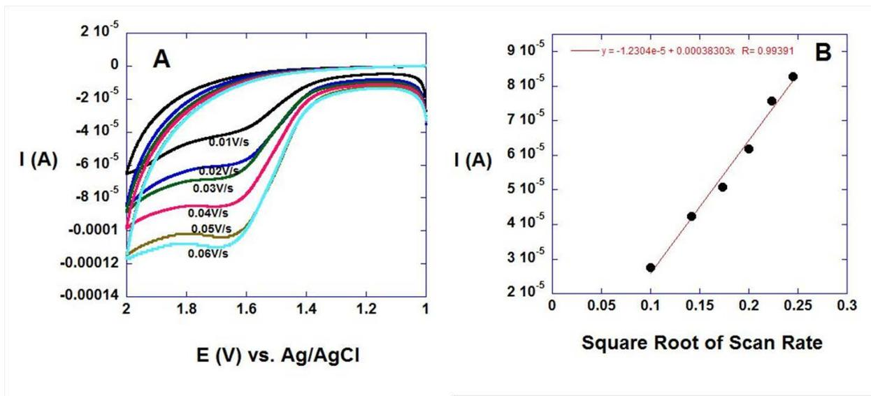
**Figure 5:** (A) Cyclic voltammograms of 0.14mM penicillin V in 0.347M SDS in ABS, pH 4.5 on glassy carbon electrode. Initial potential: 1.0V; high potential: 2.0V; low potential: 1.0V; sample interval: 0.001V, quiet time: 0.1sec. Scan rates were varied from 10mV/s to 60mV/s. (B) Calibration plot of anodic peak currents versus square root of scan rate.
