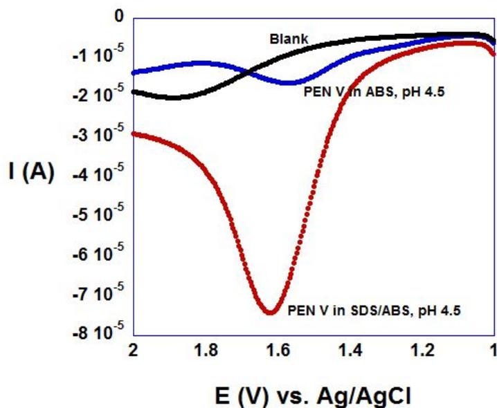
**Figure 3:** Square wave voltammograms of 0.14mM Penicillin V in ABS, pH 4.5 (Blue) and 0.14mM Penicillin V in 0.347M SDS/ABS, pH 4.5 (Red) at GC electrode. The amplitude and frequency were 0.025V and 15Hz respectively.
