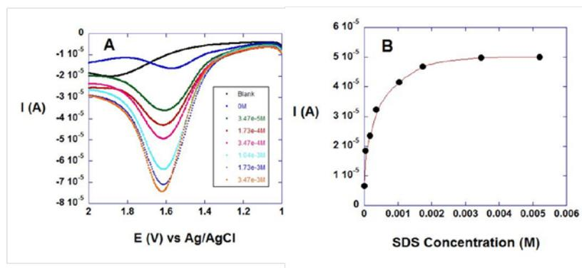
**Figure 1:** (A) Effect of successive addition of sodium dodecyl sulfate (SDS) on the voltammetric response of 0.14mM Penicillin V in ABS, pH 4.5 at GC electrode. The amplitude and frequency were 0.025V and 15Hz respectively (B) Plot of varying SDS concentrations versus voltammetric current responses.
