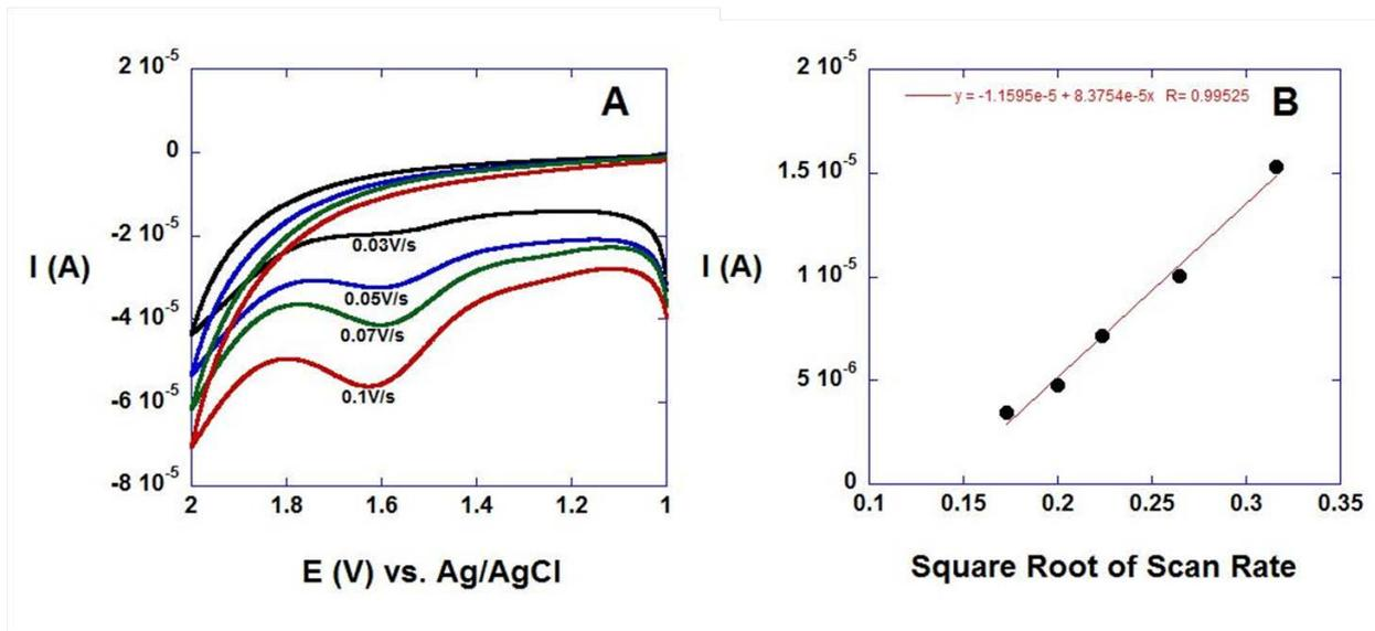
**Figure 4:** (A) Cyclic voltammograms of 0.14mM penicillin V in ABS, pH 4.5 on glassy carbon electrode. Initial potential: 1.0V; high potential: 2.0V; low potential: 1.0V; sample interval: 0.001V, quiet time: 0.1sec. Scan rates were varied from 30mV/s to 100mV/s. (B) Calibration plot of anodic peak currents versus square root of scan rate.
