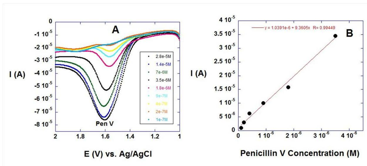
**Figure 6:** (A) Square wave voltammetry of different concentrations of Penicillin V in the SDS/ABS, pH 4.5; frequency: 15Hz and amplitude 0.025V. (B) Calibration plot of concentration of penicillin V versus voltammetric current.
