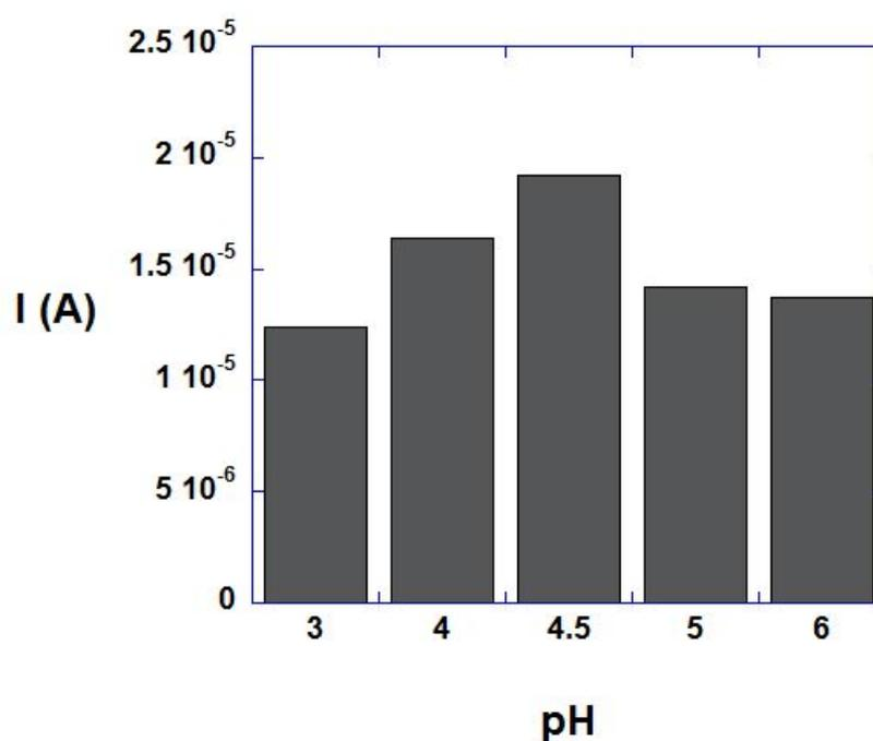
**Figure 2:** Effect of pH on the square wave voltammetric peak currents of 0.14mM Penicillin V at the GC electrode in acetate buffer. The pH values considered were 3, 4, 4.5, 5 and 6.
