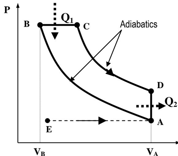
Fig. 3. P-V diagram for an ideal diesel engine
