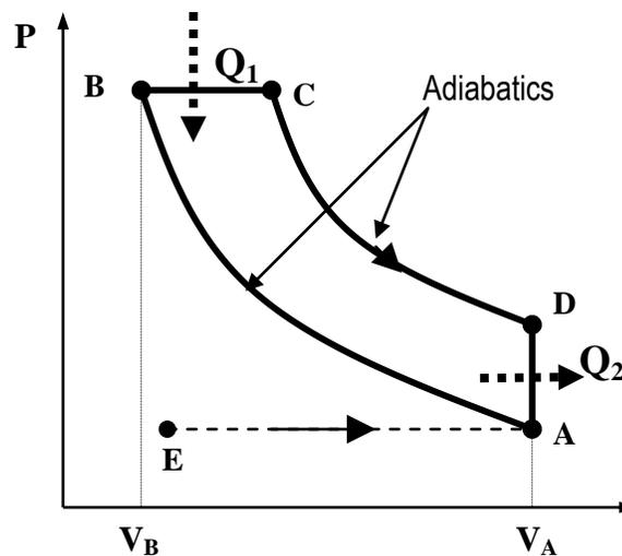
Fig. 4. P-V diagram for an ideal diesel engine
