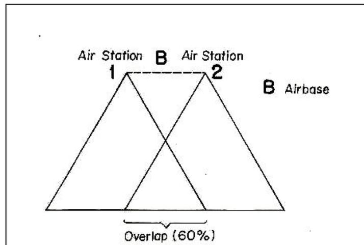
Fig. 6.2. Aerial photograph taken with an overlap of 60%.
