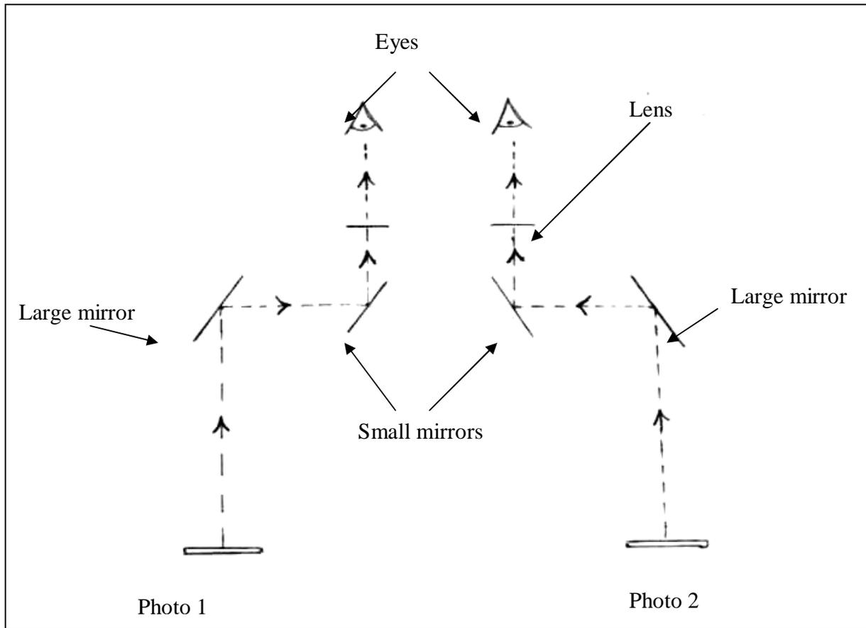
Fig. 6.5 –A sketch diagram showing the optical system of mirror stereoscopes
