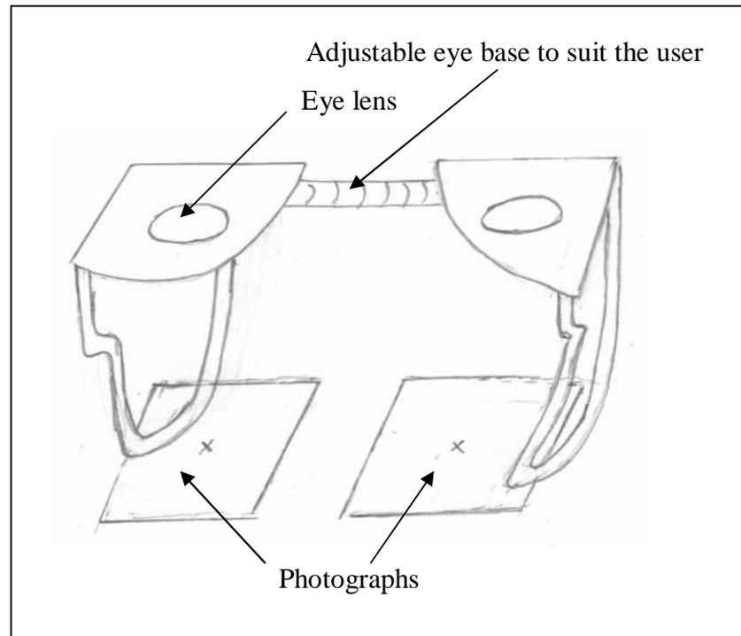
Fig. 6.4 -Simple sketch of pocket stereoscopes – 2 lenses
