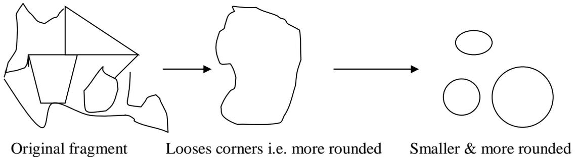
Figure 6.5 Rounding of fragments in sedimentary rocks.
