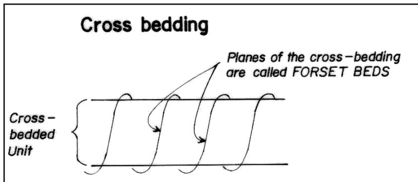
Figure 6.10 Cross-bedding structure
