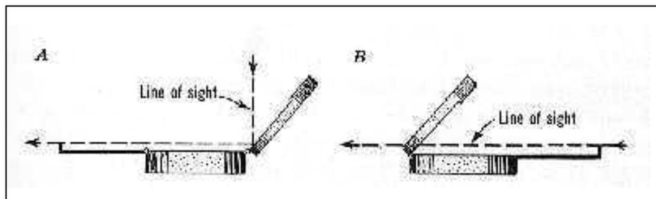
Diagram Fig.4.2A Compass set for taking a bearing at waist height (A) and at height of eye (B).
