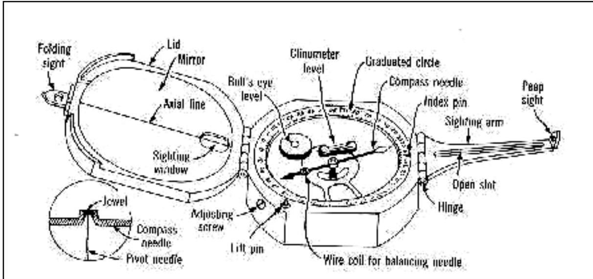
Fig. 4.1. The Brunton Compass. Inset at lower left shows enlarged section through needle bearing.
