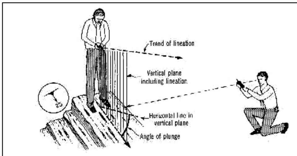
Fig. 4.4 – Measuring the trend of linear structures.
