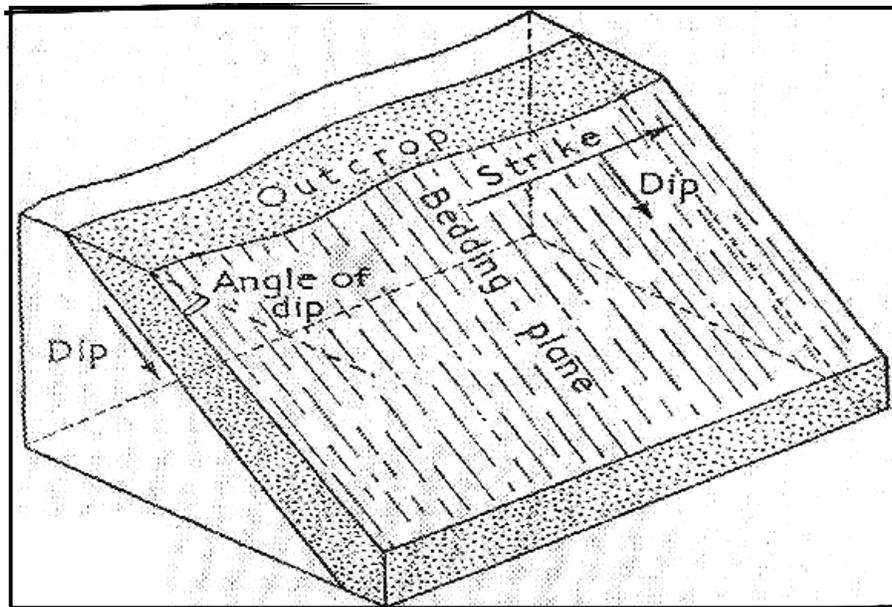
Fig. 4.3 The bedding plane, strike and dip of an inclined rock outcrop
