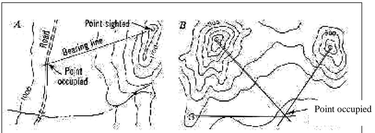
Fig. 3.2 (A). Locating a point along a road by taking a bearing to a nearby hilltop.
