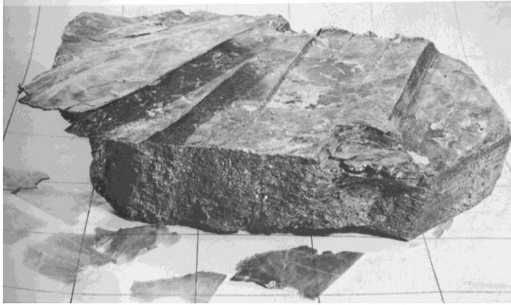
Fig. 3.1 Mica cleavage. The large block (or “book”) is bounded on the sides by crystal faces. Cleavage fragments lying in front of the large block are of different thicknesses, as indicated by their degrees of transparency.
