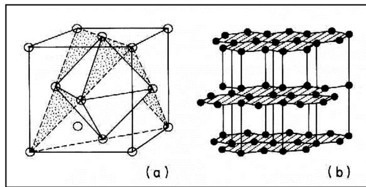
Figure 3.1. The atomic structure of diamond (a) and graphite (b).
