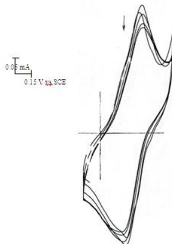
Figure 21. CV response of electrodegradation of the polyaniline and polythiophene bilayer in 0.125 M HCl. Potential limit -0.2 V to 0.86 V. Scan rate 20 mV/sec.
