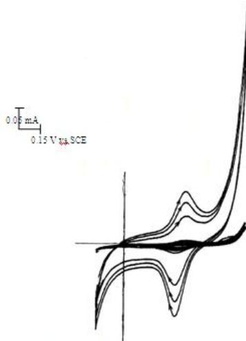
Figure 4. CV response of thiophene electrodeposited on bare carbon electrode in solution containing 0.1 M thiophene and 1 M  $H_2SO_4$ . Potential limit -0.2 V to 0.90 V. Scan rate 5 mV/sec.
