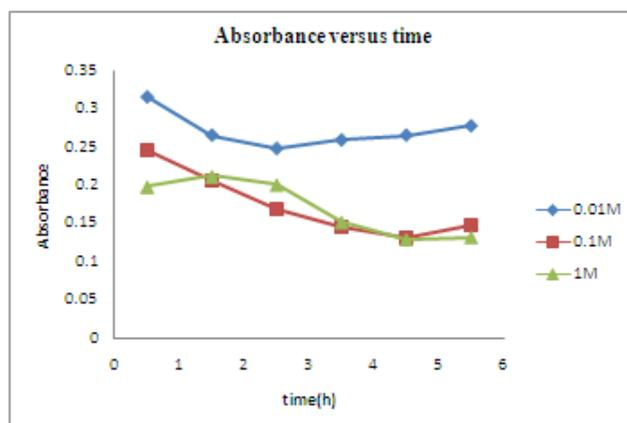
Fig. 12: Absorbances versus time for amoxicillin in 0.01M, 0.1M and 1M H<sub>2</sub>SO<sub>4</sub> solution.
