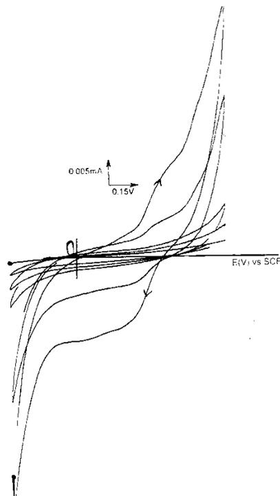
**Figure 9: CV Responses Obtained In The Case Of Amoxil/Bentonite/ Co<sup>2+</sup> Modified Electrode**
