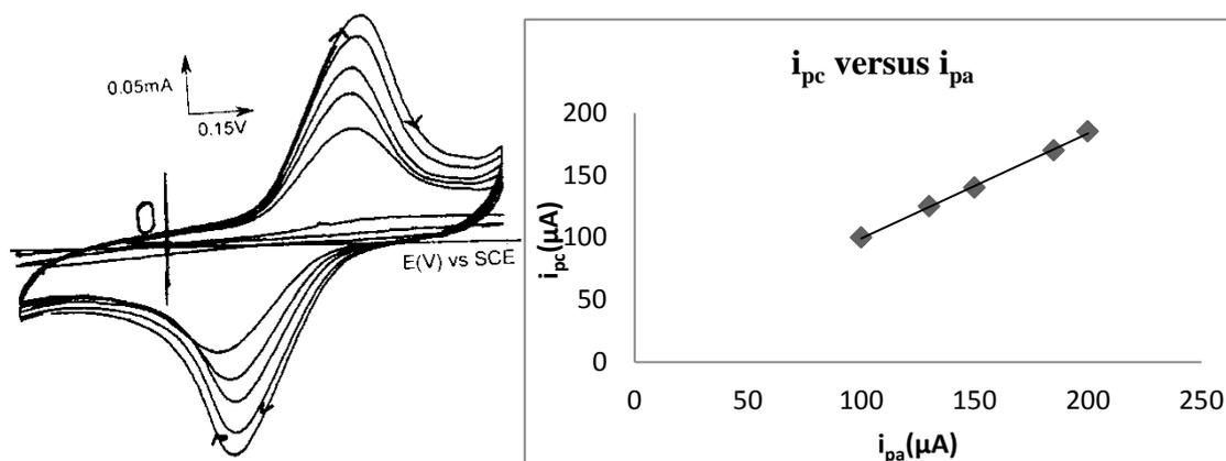
**Fig. 6: CV Responses Obtained In The Case Of Amoxil/Bentonite/Pb<sup>2+</sup> Modified Electrode**
