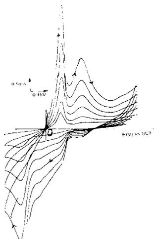
Figure 4a: CV Response Obtained In The Case Of Amoxil/Bentonite/Cu<sup>2+</sup> Modified Electrode
