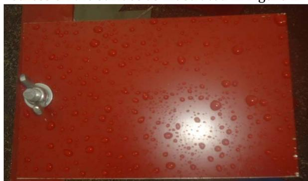
Figure 1. An installed panel showing rainfall droplets on a brick red sample at Mariakani corrosion test site, near the coastal region of Kenya
