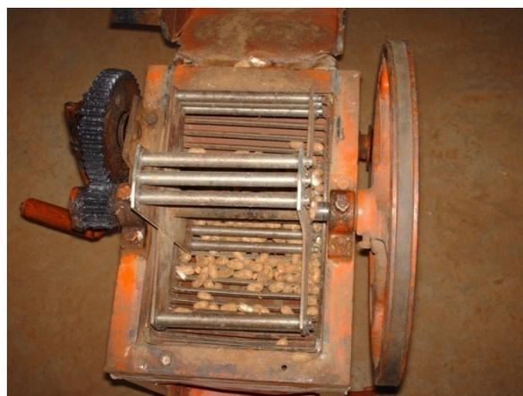
**Figure 1. Shelling unit of rod beater decorticator.**
