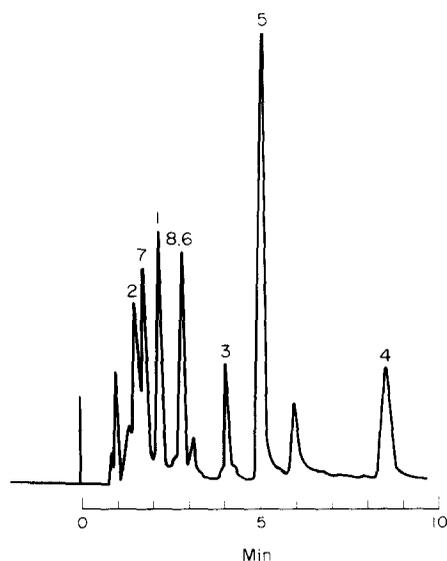
FIG. 1. HPLC PROFILE OF A CONSTITUTED MIXTURE OF SOME ANTHRAQUINONES. Column: Spherisorb ODS-2,  $3\mu$  4.6  $\times$  100 mm. Eluent: 75% acetonitrile and 25% water containing 0.01% phosphoric acid. Flow rate: 1 ml/min. Detection: UV 295 nm. Peaks: 1 knipholone; 2 islandicin; 3 chrysophanol; 4 chryslandicin; 5 physcion; 6 emodin; 7 aloë-emodinacetate; 8 chrysalodin.
