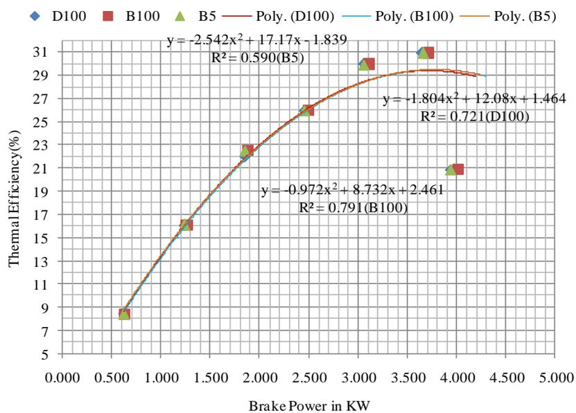
Fig 1.7 Variation of thermal efficiency with Brake power for D100, B100 and B5
