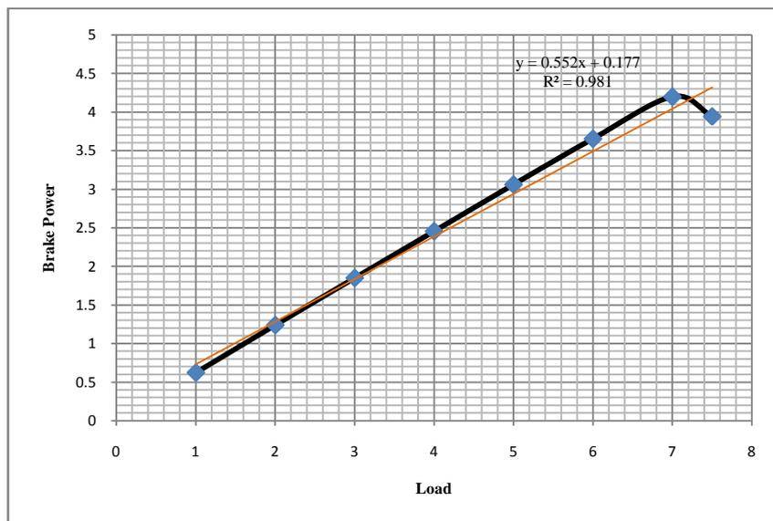
Fig 1.2 Variation of Brake Power with Load
