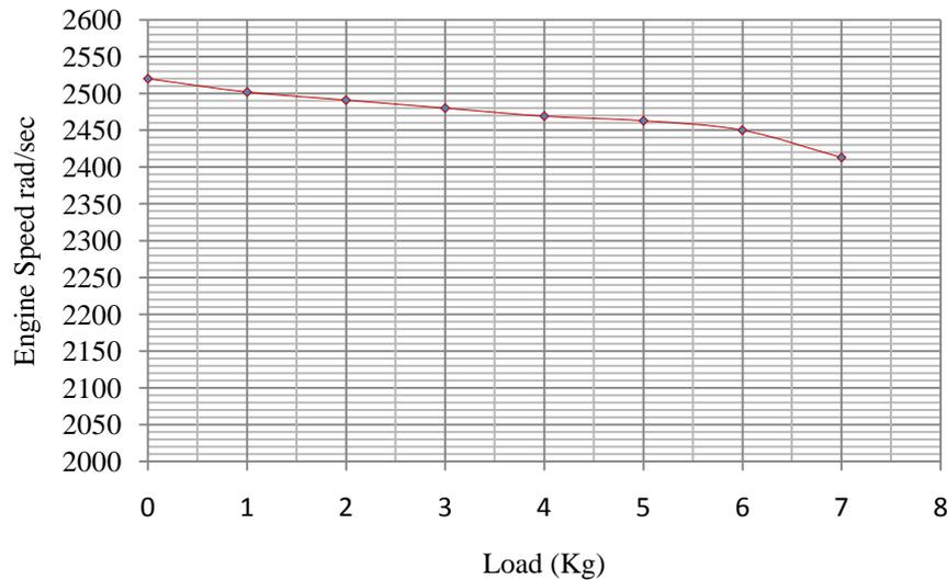
Fig 1.1 Variation of Engine Speed with Load
